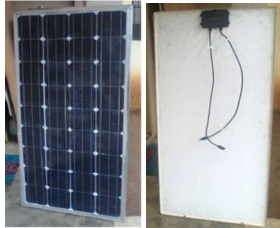
Figure 4: The constructed solar panel front and back view.
